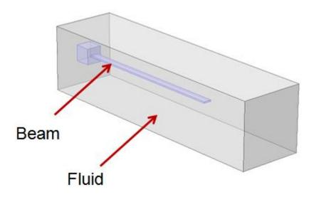
An approximate analytical solution of the form shown below is frequently used to estimate the natural frequencies of the immersed beam. This is estimated based on the *structure-only* natural frequencies, beam geometry, and the ratio of fluid-to-beam densities. The analytical expression approximately accounts for the added mass of the fluid that is displaced by the beam. It does not account for viscous effects.
